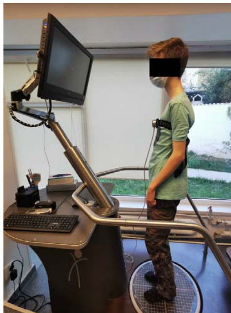
Figure 1. Advanced (computerized) stabilometry/ posturographic quantified testing and training apparatus (Pro-Kin 252), including with visual feed back (from the NTCNRCNR casuistry).
