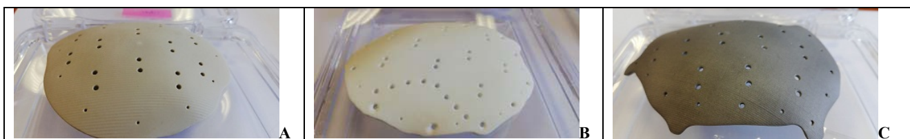
Figure 7. Implant PSI (Patient Specific Implant) from: A – PEEK , B – Bioverit II, C – Titanium 12 .
