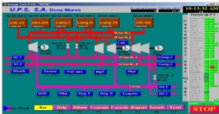
Figure 2. Main panel of the Energy Management System at Bega UPSOM thermo power station
