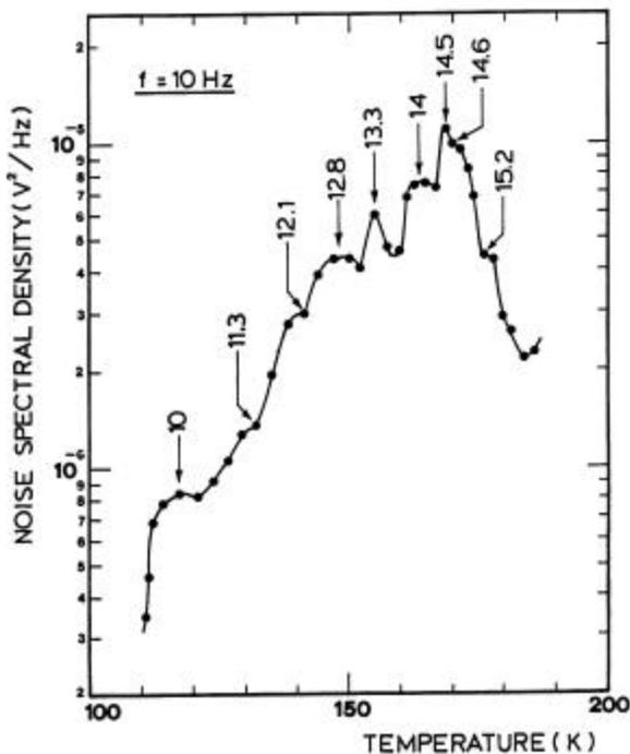
Fig. 2 - The noise spectral density ( $S_v$ ) vs. temperature. The arrows indicate the position and the corresponding energy (in meV) of each singularity in the noise.
