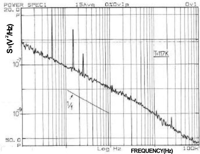
Fig.1 - The noise spectral density ( $S_v$ ) of the voltage developed across the platinum resistor terminal at 117K; this temperature corresponds to the first peak in the dependence of  $S_v$  vs. temperature (see Fig. 2).
