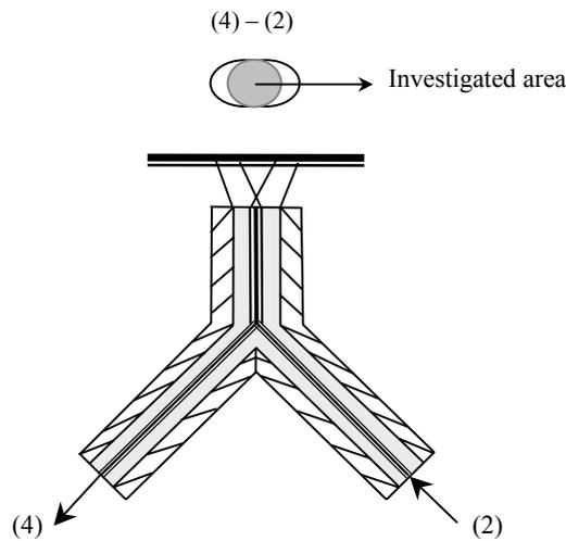
Fig. 2 Optical connector with two guiding channels
