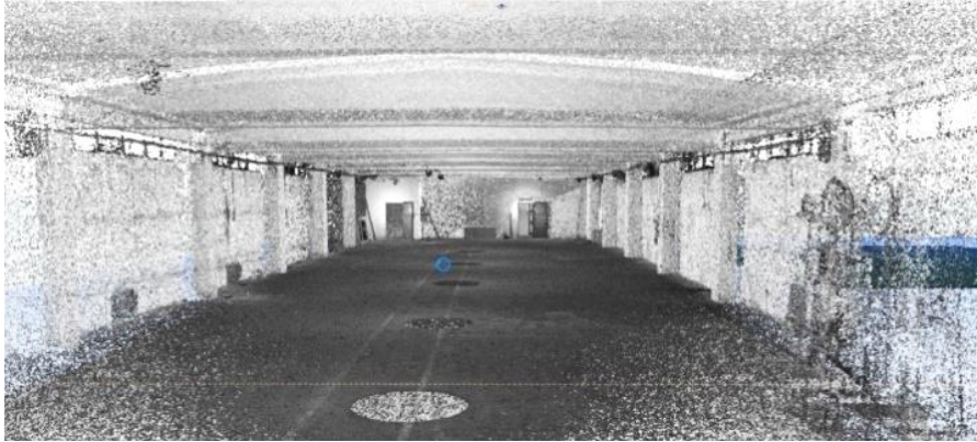
Fig. 3 – Monochrome point cloud of the interior of the building.
