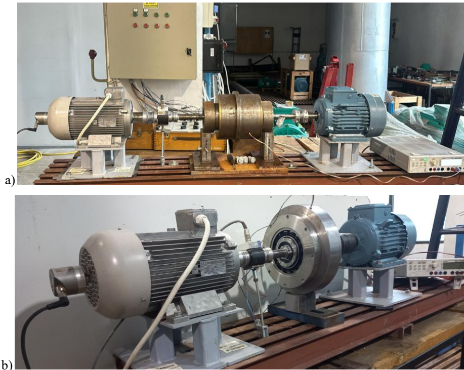
Fig. 6 – Magnetorheological clutches installed on the test rig for measuring their performances: a) MRC-CG; b) MRC-DG.
