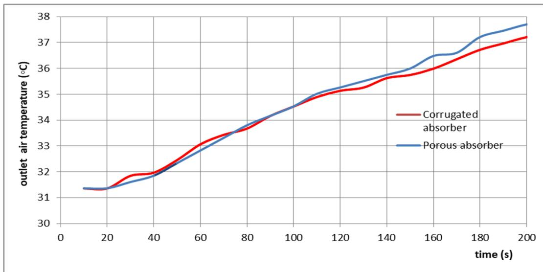
Fig. 5 – Sample experimental results – time variation for unstable solar radiative regime of the outlet air temperature corrugated collector UCAC and porous collector VPAC.
