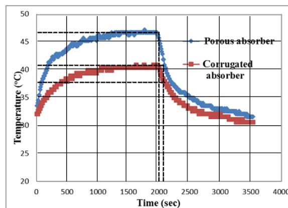
Fig. 4 – Sample experimental results of the simple shading test -time variation during a clear day of the outlet air temperature UCAC and VPAC.
