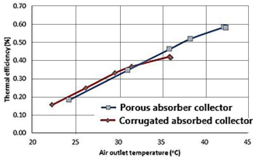
Fig. 2 – Sample experimental results showing the efficiency of the collectors as a function of outlet air temperature during clear sky days.
