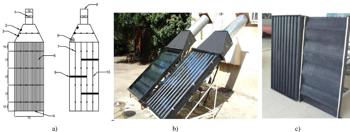
Fig. 1 – U-corrugated absorber collector (UCAC) and V-porous absorber collector (VPAC [29]):
