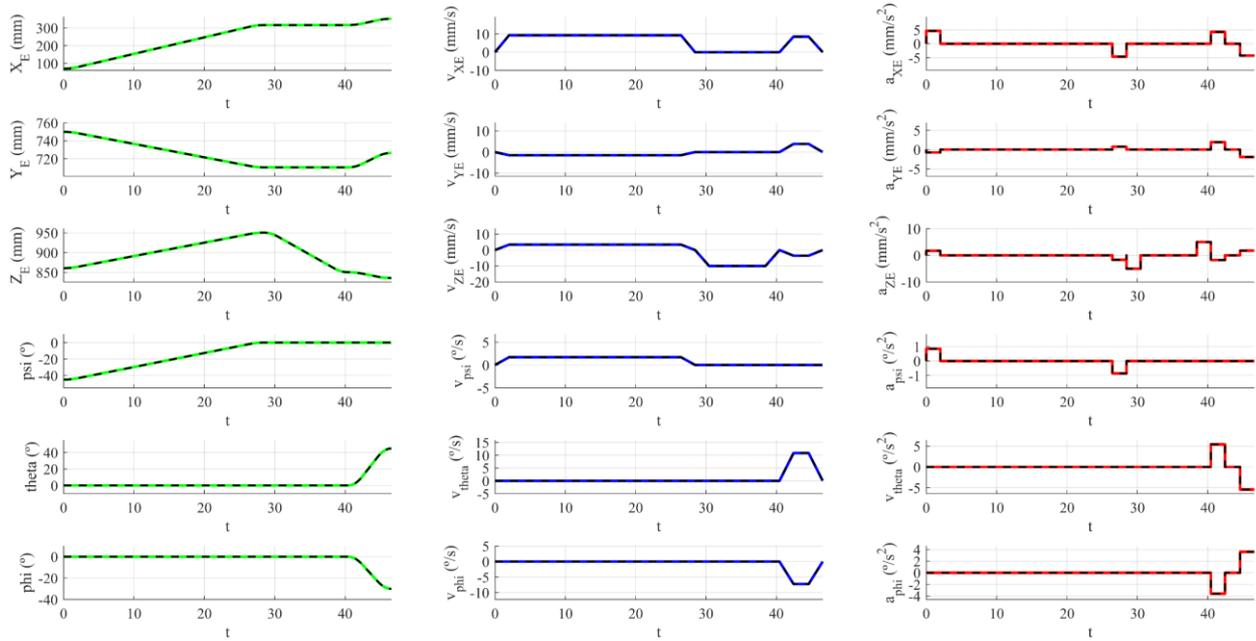
Fig. 4 – Time history diagram for the defined law of motion for the parallel robot mobile platform; green, blue, red lines (Matlab computed data); black dashed lines (Siemens NX exported data).
