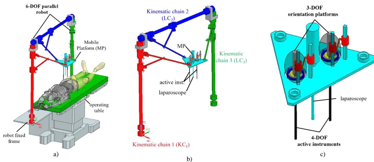
Fig 1 – CAD model of the new SILS parallel robotic system: a) parallel robotic system positioned near the operating table; b) 6-DOF parallel robot; c) mobile platform containing two 3-DOF orientation platforms for guiding the active instruments.
