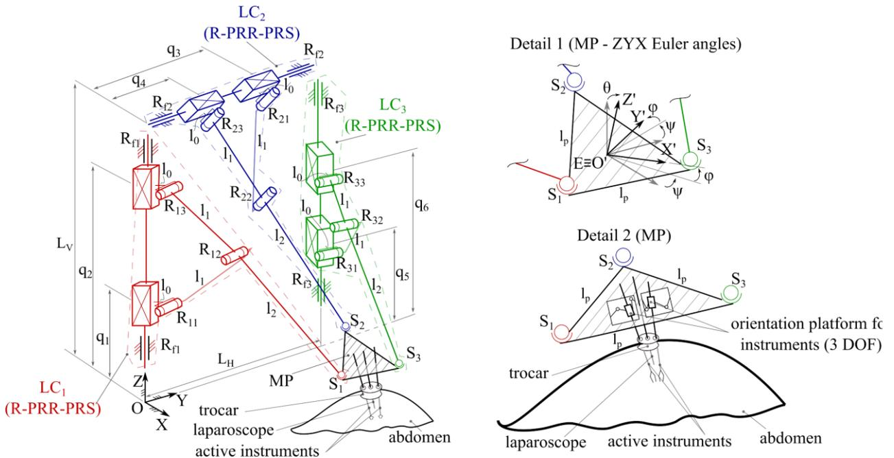
Fig. 2 – The kinematic of the parallel robotic system (type 3-R-PRR-PRS) for SILS.
