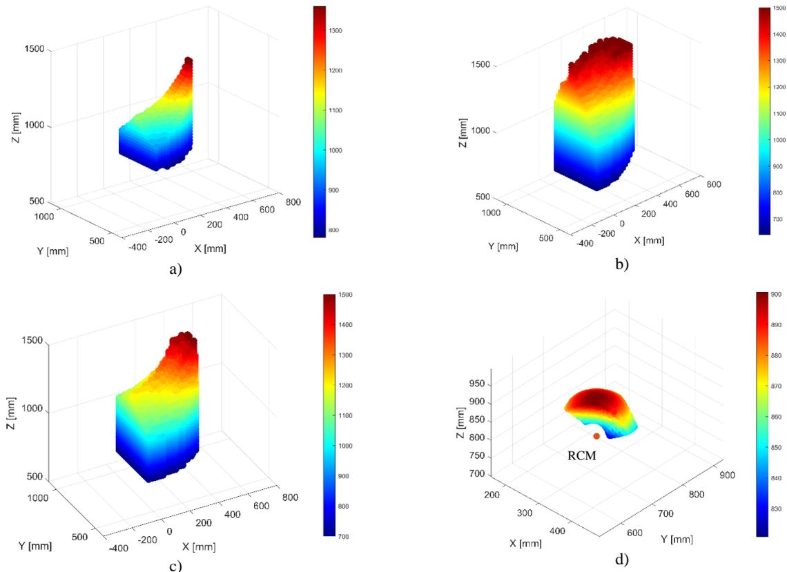
Fig. 3 – Workspace computation for the 6-DOF parallel robot for SILS.
