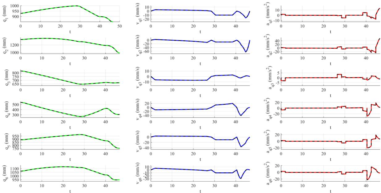
Fig. 5 – Time history diagram for the active joints of the parallel robot; green, blue, red lines (Matlab computed data); black dashed lines (Siemens NX exported data).
