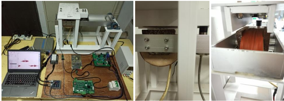
Fig. 6 – The suspension control experimental platform of the single electromagnet suspension system.
