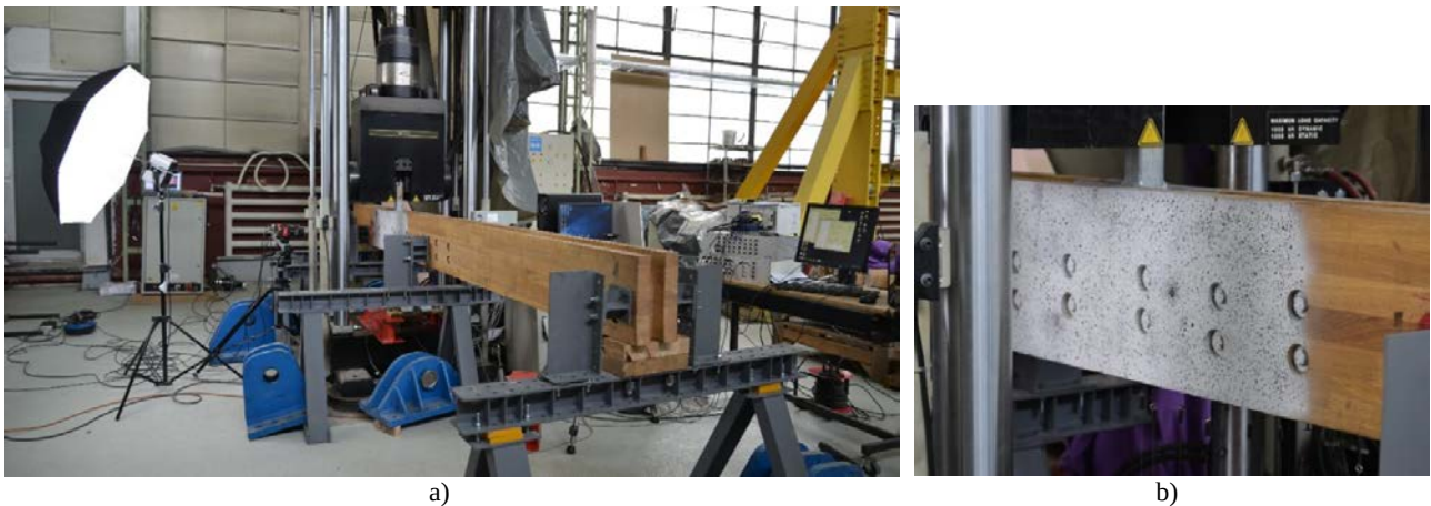
Figure 8: View from laboratory: (a) test setup and specimen ready for testing; (b) surface preparation for VIC-3D measurements
