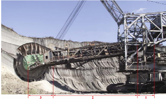
Fig. 2 – The sections of the bucket wheel's boom.
