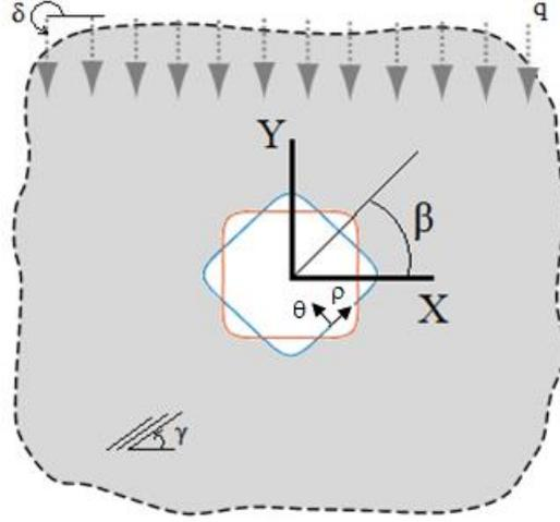
Fig. 1 – Infinite composite plate a containing quasi-square hole under uniform heat flux.
