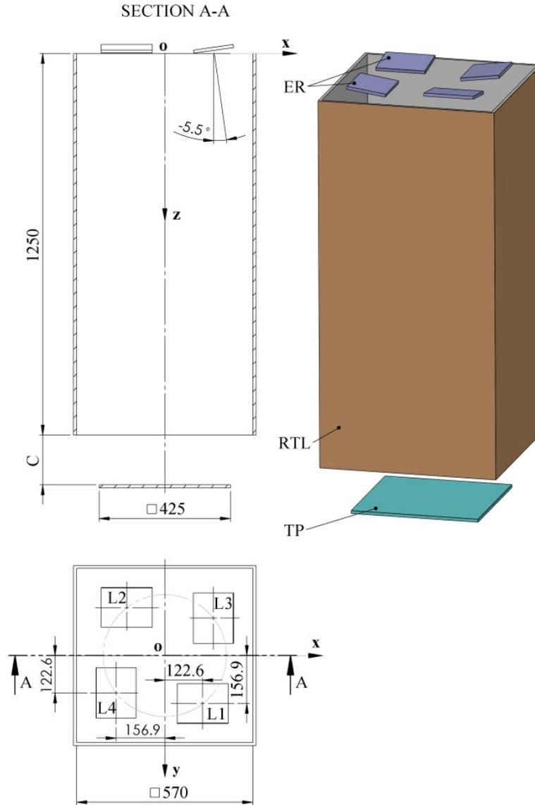
Fig. 1 – Small-scale solar simulator model for optical analysis.
