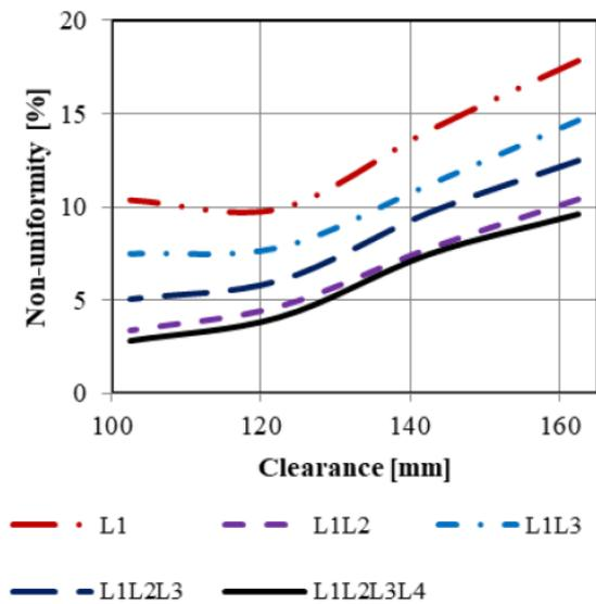
Fig. 6 – Simulated non-uniformity vs. clearance for different combinations of lit lamps.
