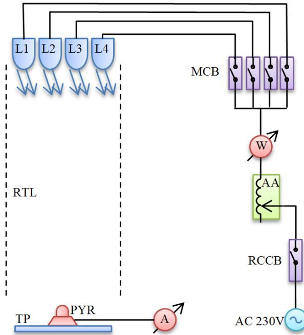
Fig. 5 – Block diagram of the small-scale solar simulator.
