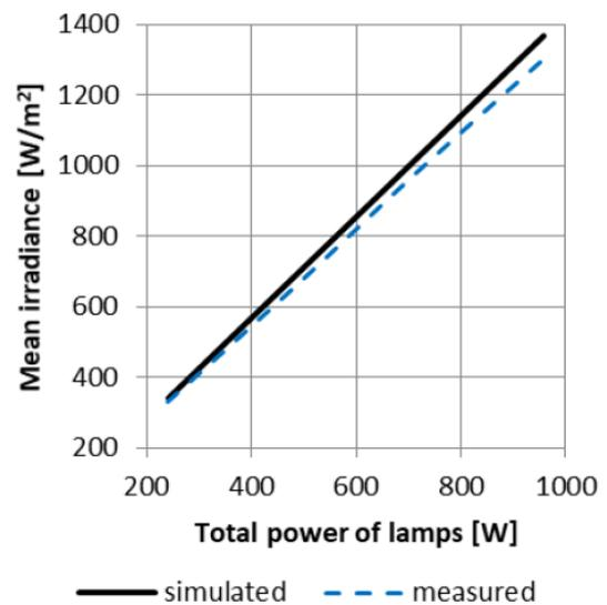
Fig. 7 – Relationship between mean irradiance and total power of lit lamps.
