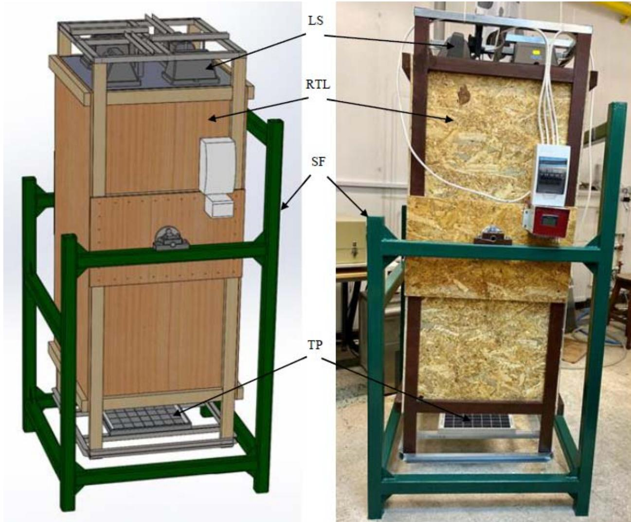
Fig. 4 – Virtual model (left) and real model (right) of the small-scale solar simulator.
