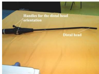
Fig. 4 – The handles used to bend the instrument head.
