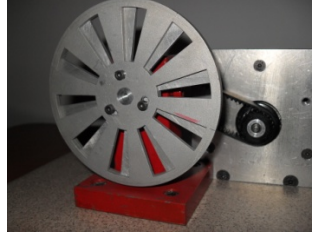
Fig. 9 – Double disk chopper [12], with the technology developed in [10].
