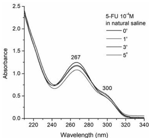
Fig. 1 – Absorption spectra of 5-FU at  $10^{-4}$  M in natural saline; pH 8.4; exposed to  $N_2$  laser radiation several irradiation times.
