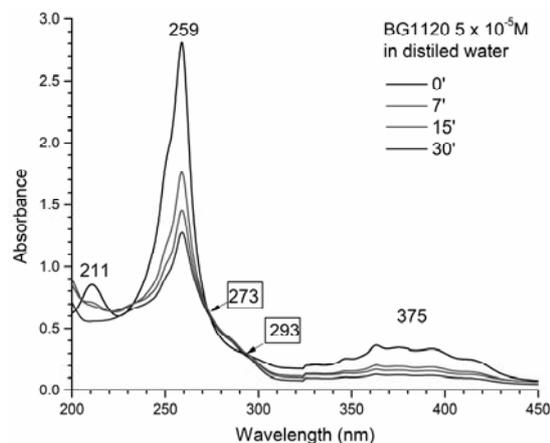
Fig. 2 – Absorption spectra of BG 1120,  $5 \times 10^{-5}$  M solutions in distilled water for several irradiation times, using cw Xe lamp.
