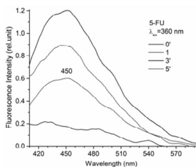
Fig. 4 – Fluorescence emission spectra of 5-FU solutions exposed to  $N_2$  laser radiation.
