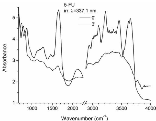
Fig. 8 – FTIR spectrum of 5-FU for unirradiated compared to 3 min laser irradiated solution at 337.1 nm.
