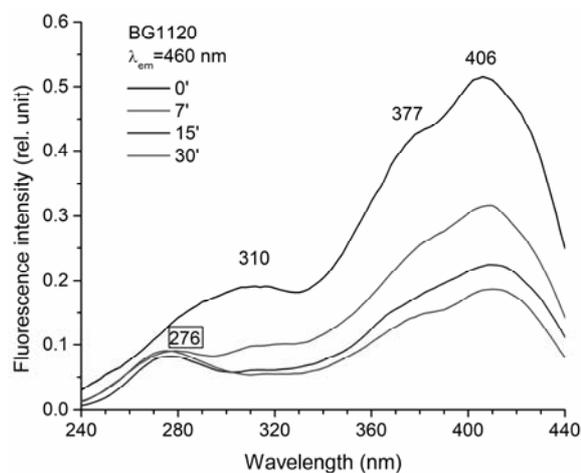
Fig.7 – Fluorescence excitation spectra of BG 1120 solutions  $5 \times 10^{-5}$  M in distilled water for several irradiation times with cw Xe lamp;  $\lambda_{\text{em}} = 460$  nm.
