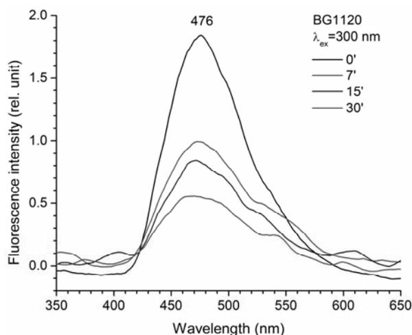
Fig. 6 – Fluorescence emission spectra of BG 1120 solutions,  $5 \times 10^{-5}$  M in distilled water for several irradiation times with cw Xe lamp;  $\lambda_{\text{ex}} = 300$  nm.
