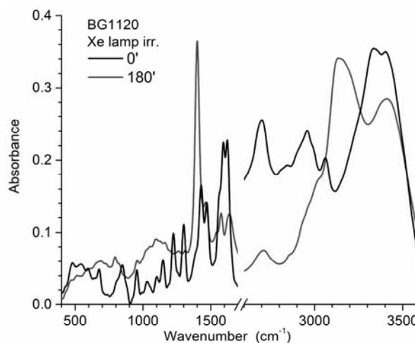
Fig. 9 – FTIR spectra of unirradiated and 180 min irradiated BG 1120 solution in distilled water with a cw Xe lamp.
