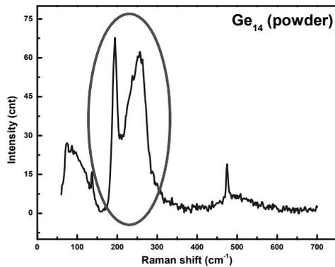
Fig. 3 – Raman spectra of  $Ge_{0.14}As_{0.14}Se_{0.72}$  powder samples.
