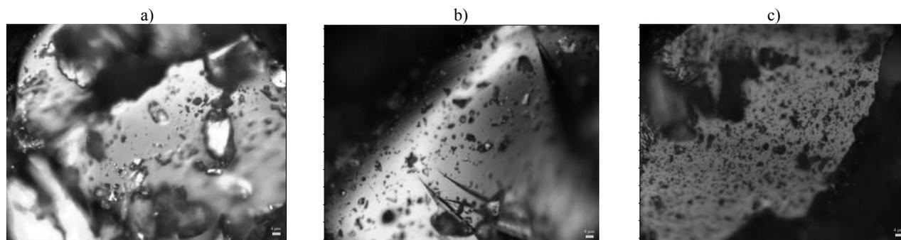
Fig. 9 – a) The area where the Raman spectrum of  $\text{Ge}_x\text{As}_x\text{Se}_{1-2x}$  samples was recorded (magnification –  $50\times$ ). Composition  $x$ : a)  $x = 0.05$ ; b)  $x = 0.16$  (b); c)  $x = 0.30$ .
