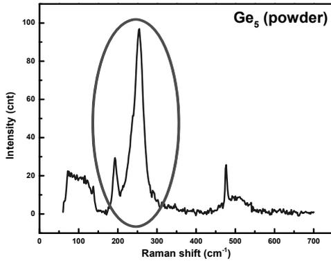
Fig. 1 – Raman spectra of  $Ge_{0.05}As_{0.05}Se_{0.90}$  powder samples.
