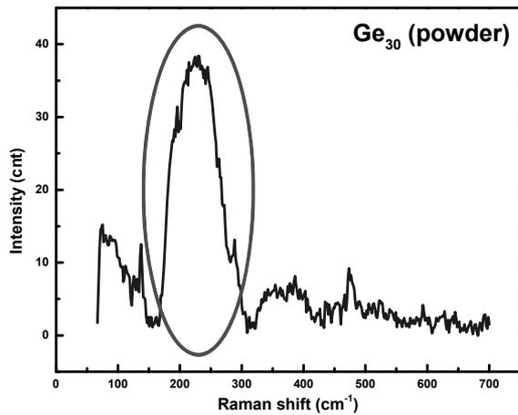
Fig. 5 – Raman spectra of  $\text{Ge}_{0.30}\text{As}_{0.30}\text{Se}_{0.40}$  powder samples.
