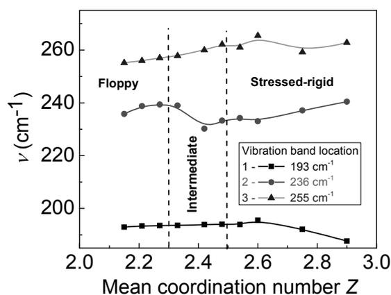
Fig. 8 – Dependence of the position of the peaks of main vibration bands ( $\nu = 193 \text{ cm}^{-1}$ ,  $\nu = 236 \text{ cm}^{-1}$ , and  $\nu = 255 \text{ cm}^{-1}$ ) in the Raman spectra of  $\text{Ge}_x\text{As}_x\text{Se}_{1-2x}$  powder samples.
