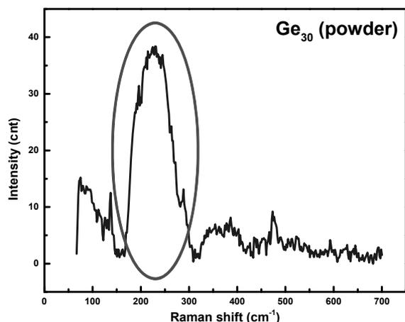
Fig. 5 – Raman spectra of  $\text{Ge}_{0.30}\text{As}_{0.30}\text{Se}_{0.40}$  powder samples.
