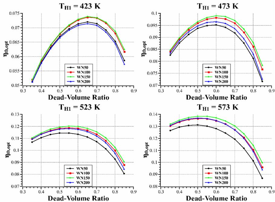
Fig 2 – Thermal efficiency *versus* dead-volume ratio at the four different source temperatures.
