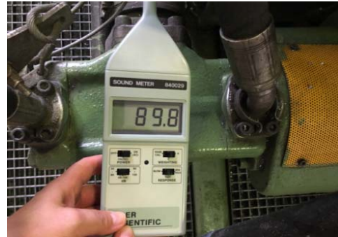
Fig. 11 – Measurement noises near pump of machine.
