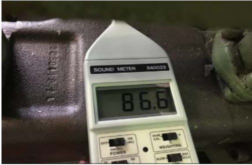
Fig. 10 – Sonometer equipment use to noises measurements.
