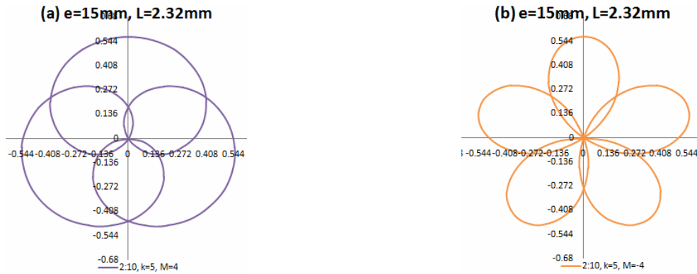
Fig. 9 – Ascertainment of the necessary distance L from the scanner to the screen in order to obtain scan patterns that pass through the O.A./z-axis ( i.e. , through the geometrical center of the scan pattern), for: a) M = 4 ; b) M = 4 (both with k = 5 , value obtained with a pair of prisms with prisms angles of 2^\circ and 5^\circ , respectively).
