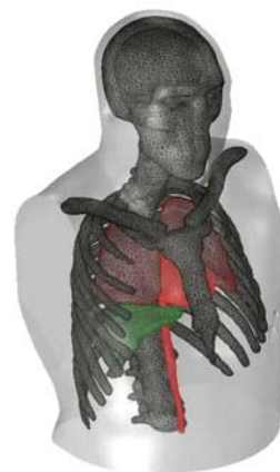
b) FEM mesh, made of approximately 565,000 tetrahedral elements.
