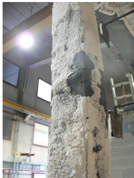
Fig. 3 – Local buckling during test.
