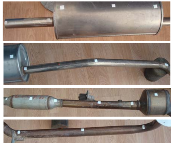
Fig. 9 – Impact locations on the structure.
