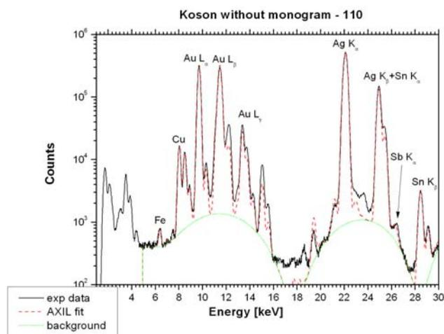
Fig. 10 – Koson without monogram – micro-SR-XRF spectrum.
