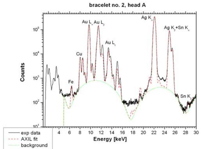
Fig. 5 – Dacian bracelet no. 2, head A – micro-SR-XRF spectrum.
