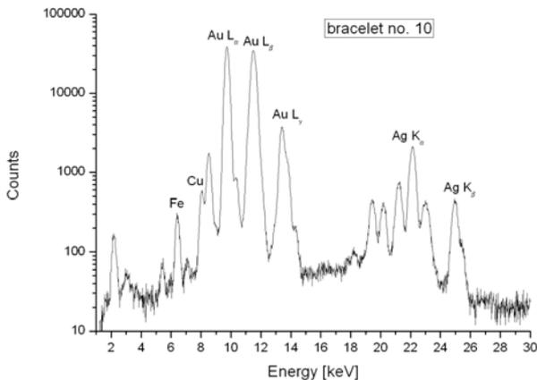
Fig. 4 – Dacian bracelet no.10 – XRF spectrum.
