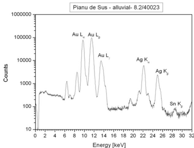
Fig. 12 –Alluvial gold, Lupsa, Valea Ariesului- micro-SR-XRF spectrum. Fig. 13 –Alluvial gold, Pianul de Sus- micro-SR-XRF spectrum.
