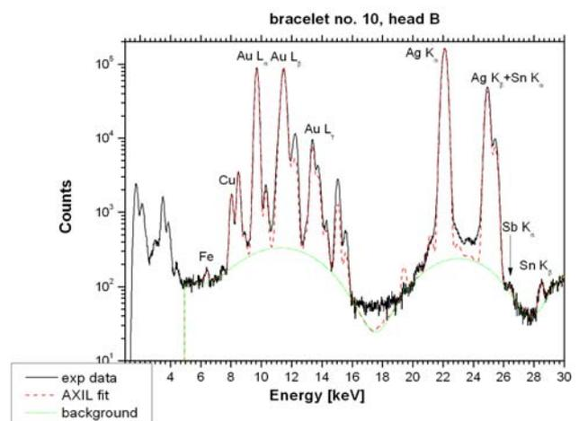
Fig. 7 – Dacian bracelet no. 10, head B – micro-SR-XRF spectrum.
