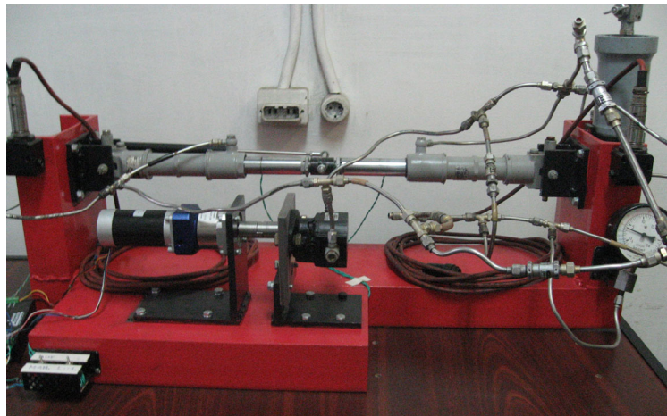
Fig. 6 – View of the test rig for the hydrostatic actuator.
