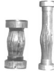
Fig. 7  $\sigma_1 - \sigma_2$  complex stress state in a uniaxial compression test.
