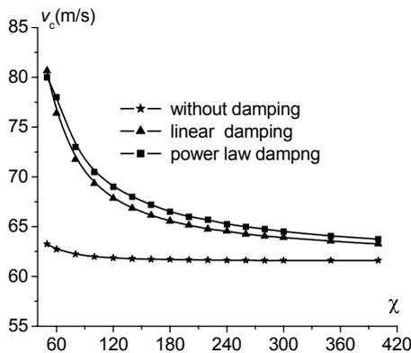
Fig. 14 – The variation of critical speed for stable regimes of the hunting motion.
