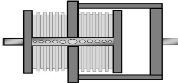
Fig. 3 – Hydraulic nonlinear devices with metal bellows.
