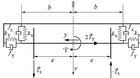
Fig. 1 – The mechanical model of wheelset with elastic joints.
