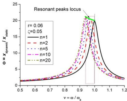
Fig. 5.5 – Magnification functions for different number of cycles under  $r = 0.06$  and  $\zeta = 0.05$ .
