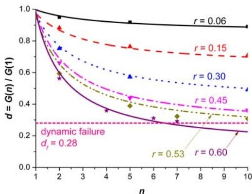
Fig. 3.1 – Some degradation functions for clay.
