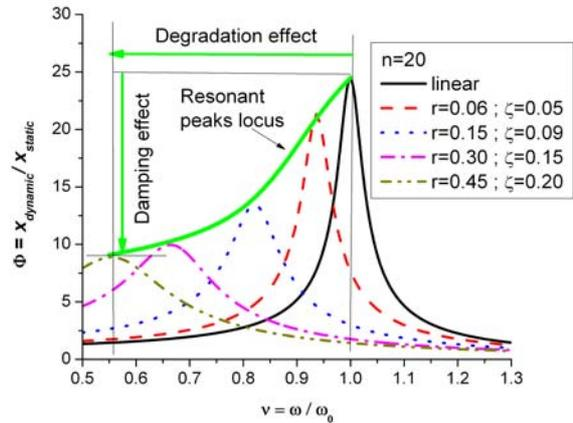
Fig. 5.4 – Magnification functions for the 20<sup>th</sup> cycle.
