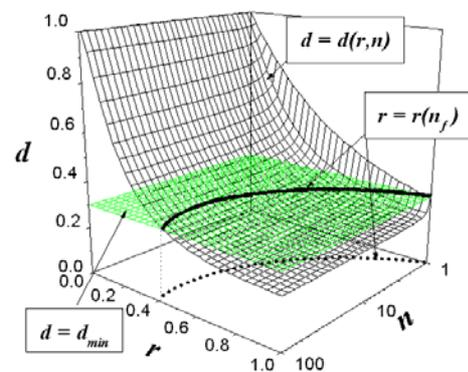
Fig. 3.2 – Spatial diagram of the degradation function.
