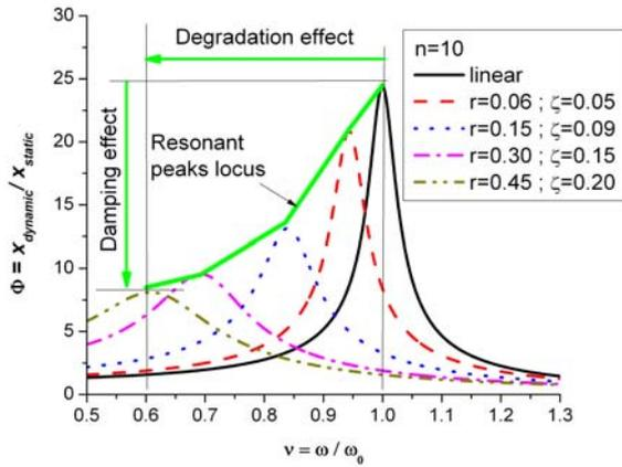
Fig. 5.3 – Magnification functions for the 10<sup>th</sup> cycle.
