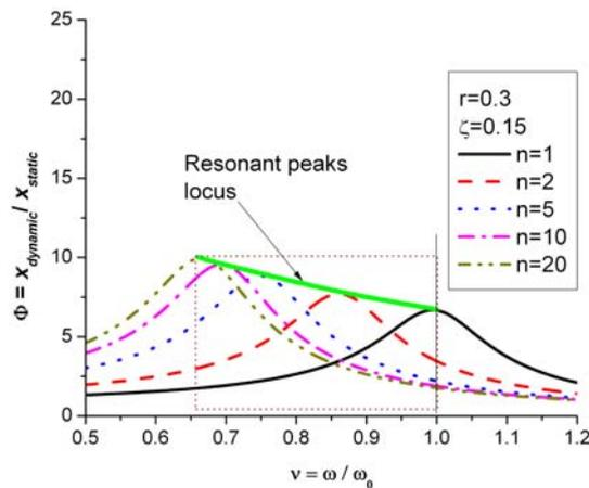
Fig. 5.7 – Magnification functions for different number of cycles under  $r = 0.3$  and  $\zeta = 0.15$ .
