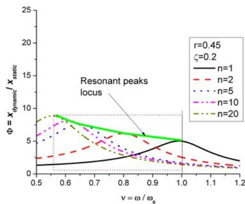
Fig. 5.8 – Magnification functions for different number of cycles under  $r = 0.45$  and  $\zeta = 0.2$ .
