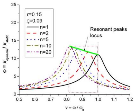
Fig. 5.6 – Magnification functions for different number of cycles under  $r = 0.15$  and  $\zeta = 0.09$ .
