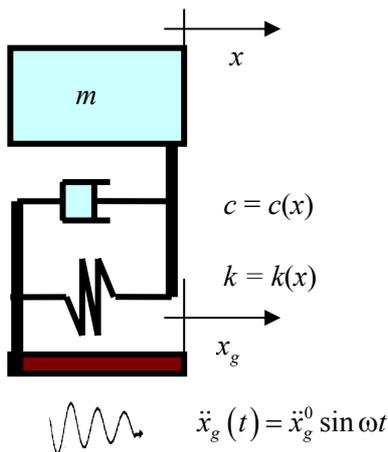
Fig. 4.1 – NKV model with abutment excitation.
