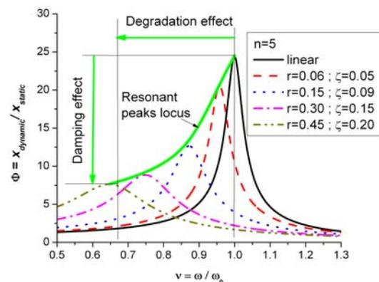
Fig. 5.2 – Magnification functions for the 5<sup>th</sup> cycle.
