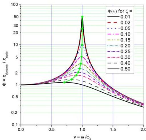
Fig. 2.1 – Linear magnification functions.
