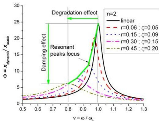
Fig. 5.1 – Magnification functions for second cycle.
