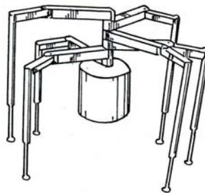
Fig. 1 – Walking vehicle with weaving gait.
