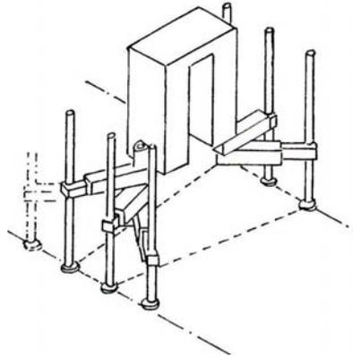
Fig. 2 – Walking robot with circular gait.
