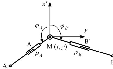
Fig. 8 – Kinematic propulsive chain, type RTRTR.
