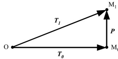
Fig. 4 – The graph of homogeneous transformation for an elementary displacement on a straight line.
