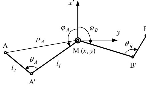
Fig. 7 – The propulsive mechanism chain, type RRRRR.
