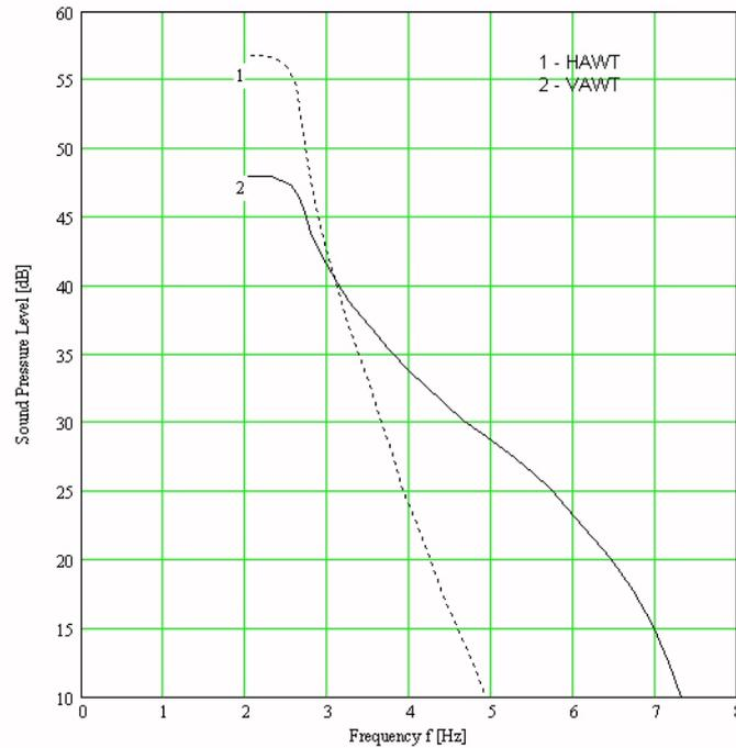
Fig. 6 – Computed spectra for the horizontal and vertical rotors.
