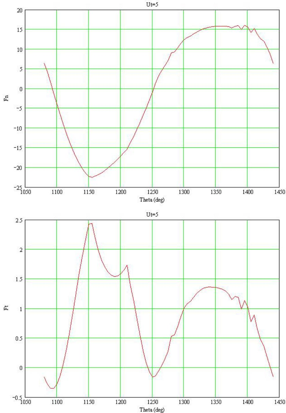
Fig. 4 – Distribution of normal and tangential forces at  $\lambda=5$ .
