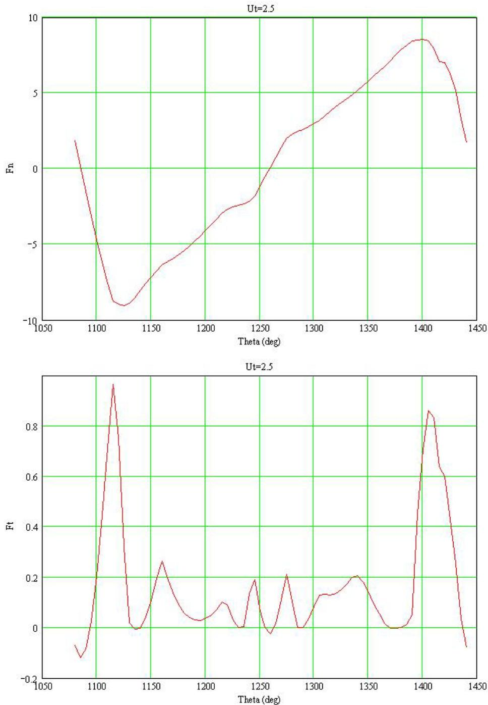
Fig. 3 – Distribution of normal and tangential forces at  $\lambda=2.5$ .
