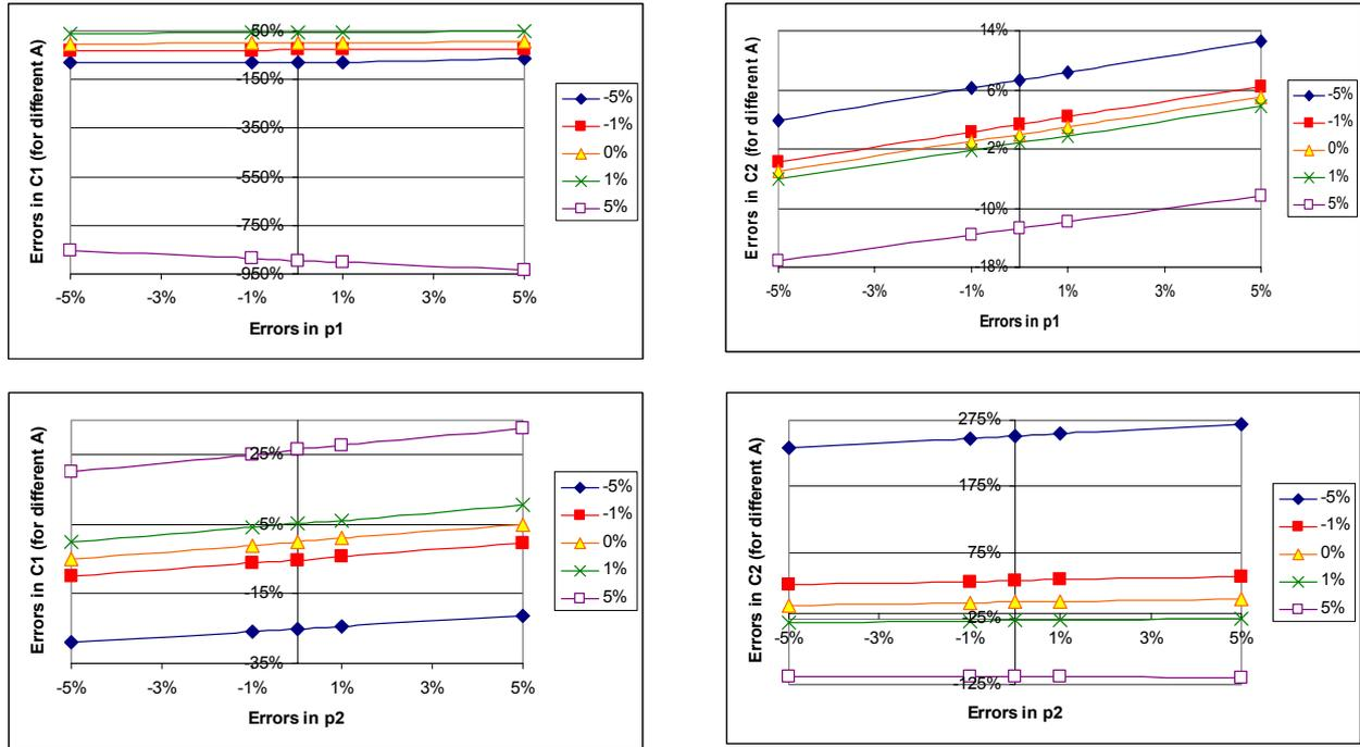
Fig. 2 – Percent errors for constants  $C_1$  and  $C_2$ , for up to 5% errors in  $A=10.5189$  cm and  $p_1 = -10.0123$  kg f/ cm<sup>2</sup> (Case 1.1, top) and  $p_2 = 6.8956$  kg f/ cm<sup>2</sup> (Case 1.2, bottom).
