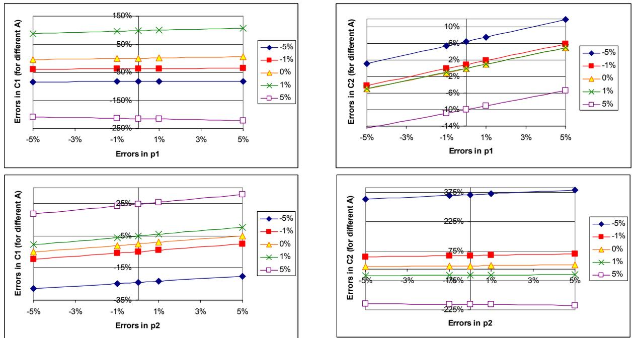
Fig. 3 – Percent errors for constants  $C_1$  and  $C_2$ , for up to 5% errors in  $A = 10.7222$  cm and  $p_1 = -10.2112$  kg f/ cm<sup>2</sup> (Case 2.1, top) and  $p_2 = 14.1934$  kg f/ cm<sup>2</sup> (Case 2.2, bottom).
