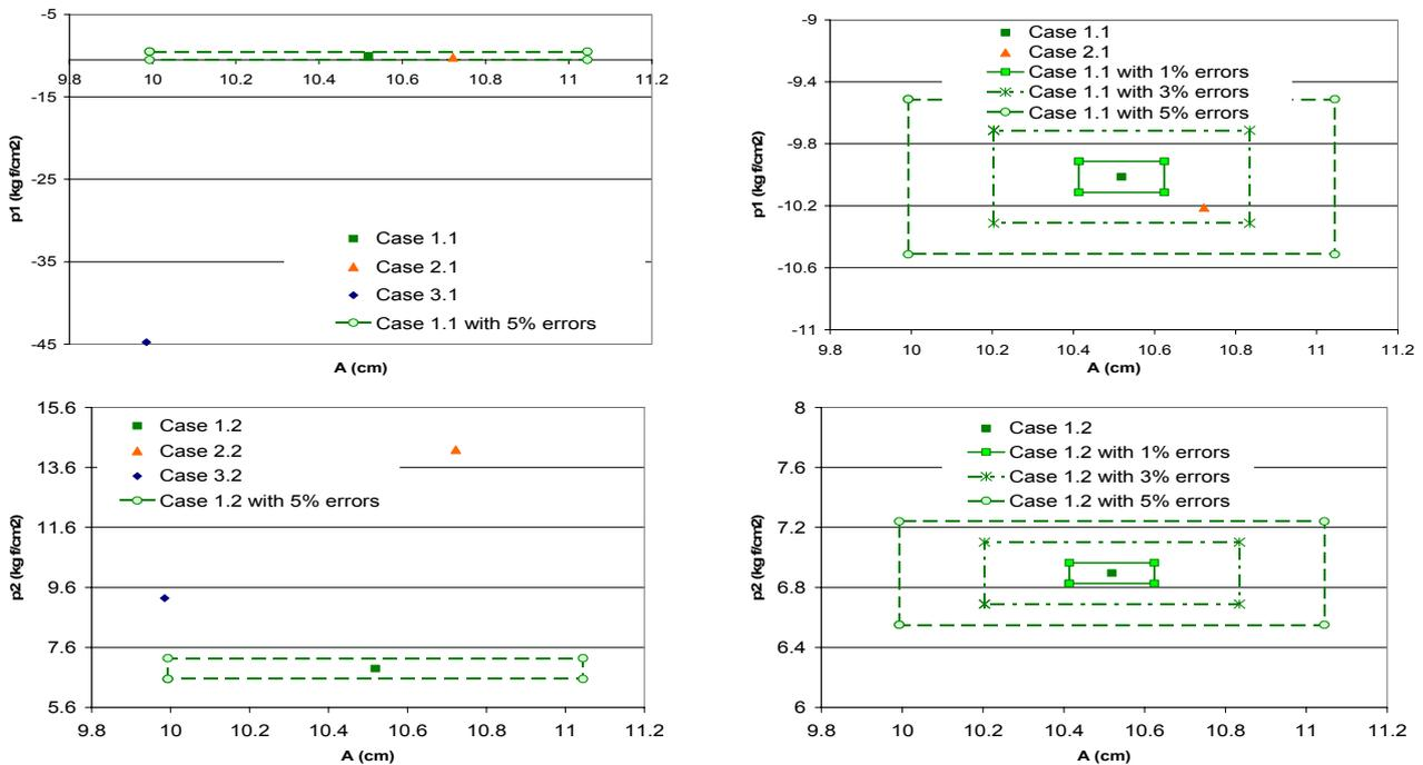
Fig. 5 – Representation of the three cases in the eversion constant-pressure space. When the couple  $A - p_1$  is measured as input for the inverse problem, cases 1-2 cannot be distinguished with measurement errors of 2% or more; the same relative error have no confounding effect on the three cases represented in the space  $A - p_2$ . Figures on right are zoom-in of figures on the left.
