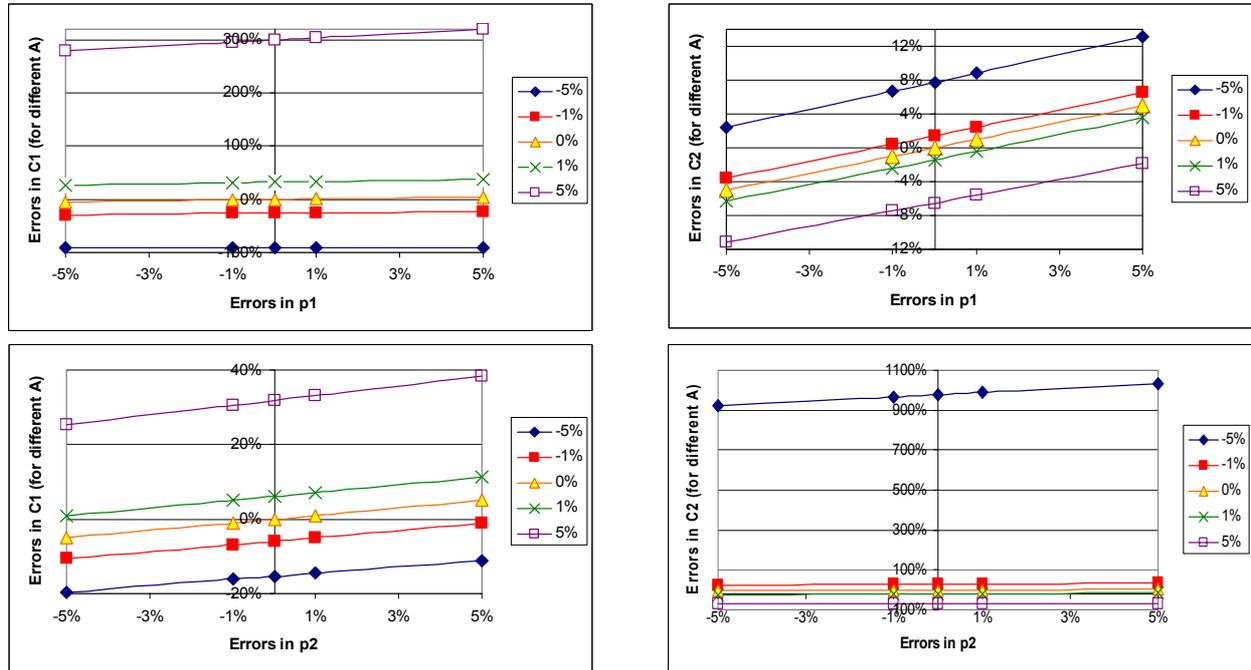
Fig. 4 – Percent errors for constants  $C_1$  and  $C_2$ , for up to 5% errors in  $A = 9.9848$  cm and  $p_1 = -44.7483$  kg f/cm<sup>2</sup> (Case 3.1, top) and  $p_2 = 9.2477$  kg f/cm<sup>2</sup> (Case 3.2, bottom).
