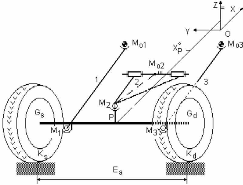
Fig. 4. The structural model for the 2S1C guiding mechanism of the rear axle.
