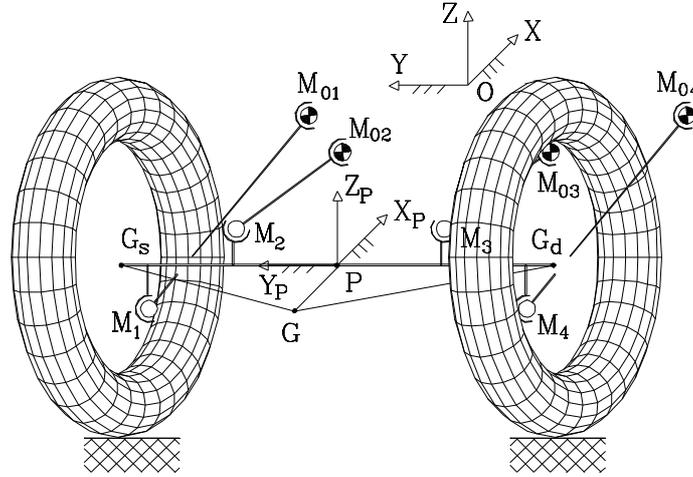
Fig. 2. The global and local reference frames for the rear suspension system.
