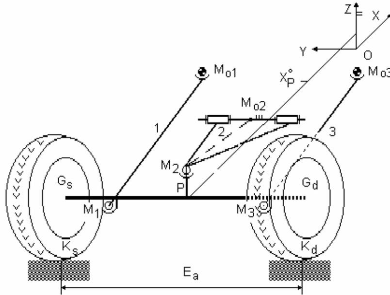
Fig. 4. The structural model for the 2S1C guiding mechanism of the rear axle.
