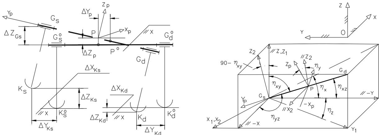
Fig. 3. The kinematic functions (parameters) of the rear axle.
