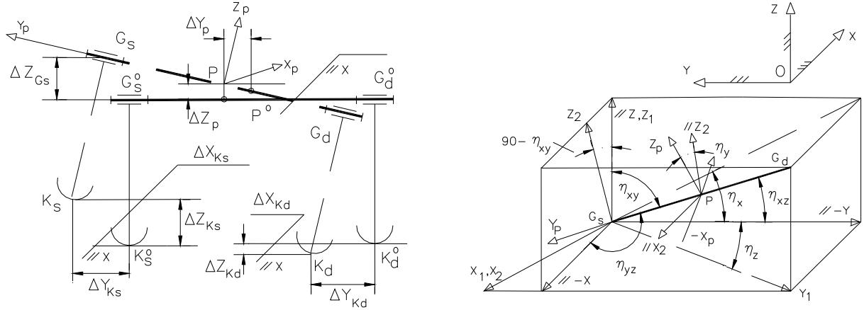
Fig. 3. The kinematic functions (parameters) of the rear axle.
