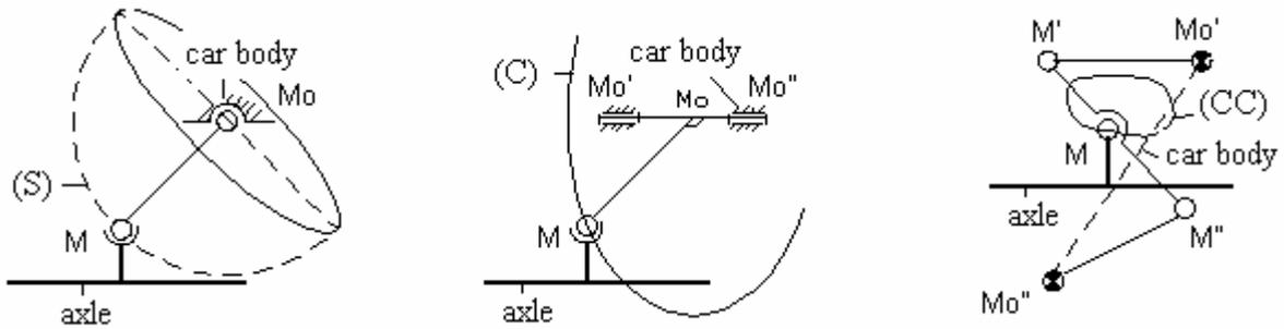
Fig.1. The basic types of guidance of the rear axle.
