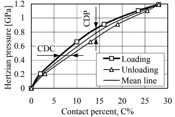
Figure A.2. Load influence on film contact (reversed axes)
