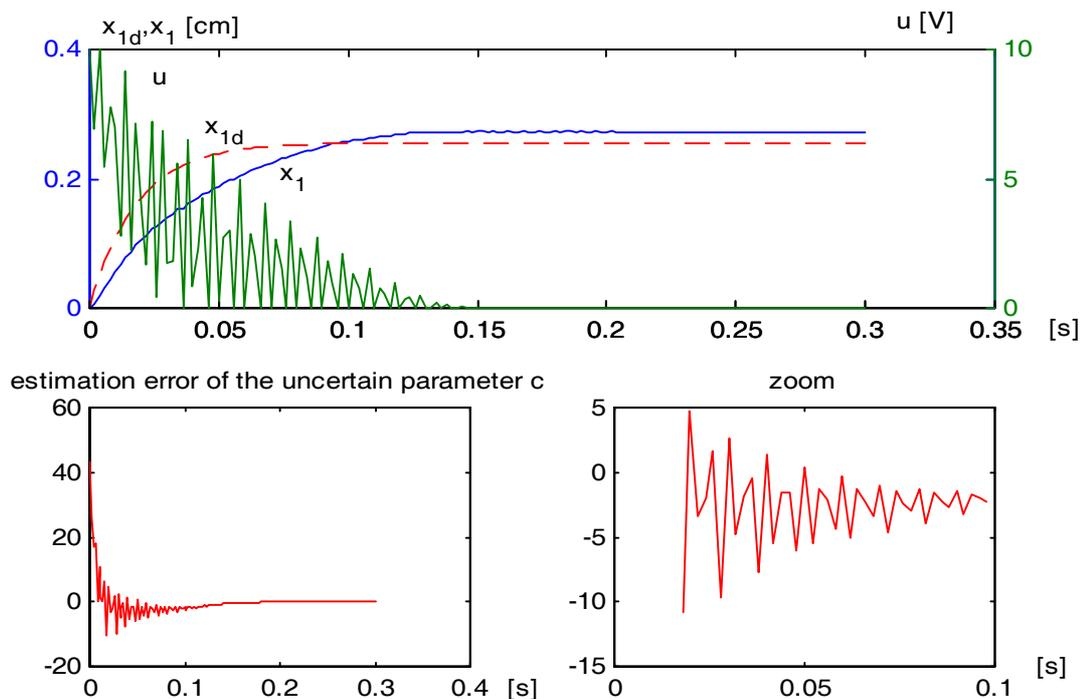
Fig. 3 – Robustness of system in Fig. 1 versus  $\tau$  maximal admissible value: performance worsened somewhat,  $\tau_c \cong 0.042$  s.
