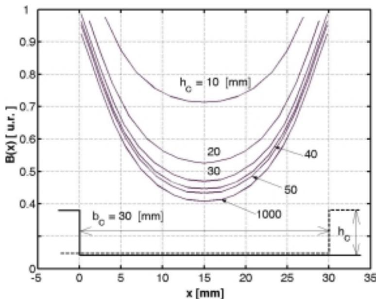
Fig. 3. The field solution for  $b_c = 30$  mm and different slot heights:  $h_c = 10$  mm, 20 mm, 30 mm, 40 mm, 50 mm, 1000 mm.
