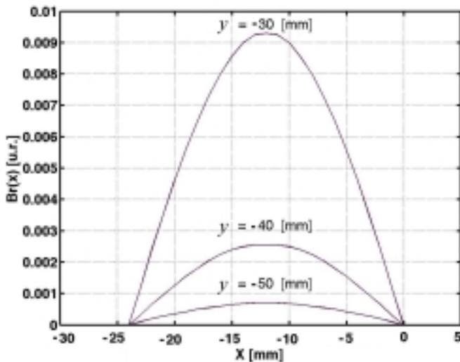
Figure 6. The distribution of the flux density radial component for larger depths:  $y=-30$  mm;  $y=-40$  mm;  $y=-50$  mm.
