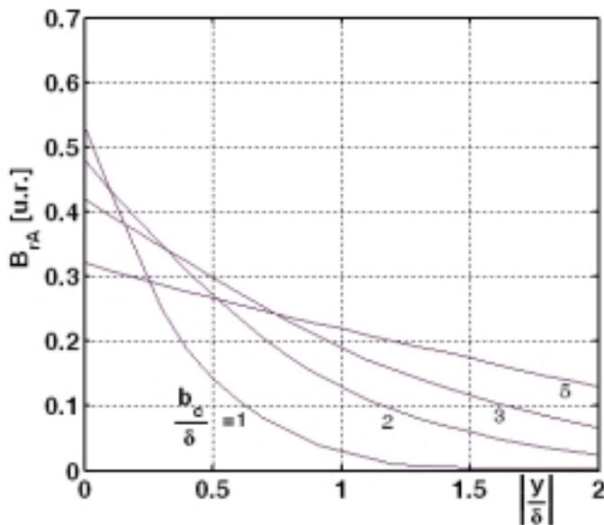
Fig. 7 The variation of the flux density radial component in the slot axe (near the air gap)
