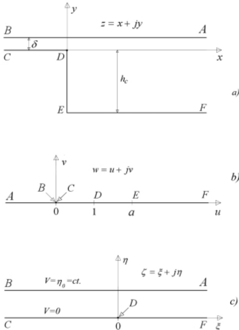
Fig.1 The conformal mapping of the complex planes:
