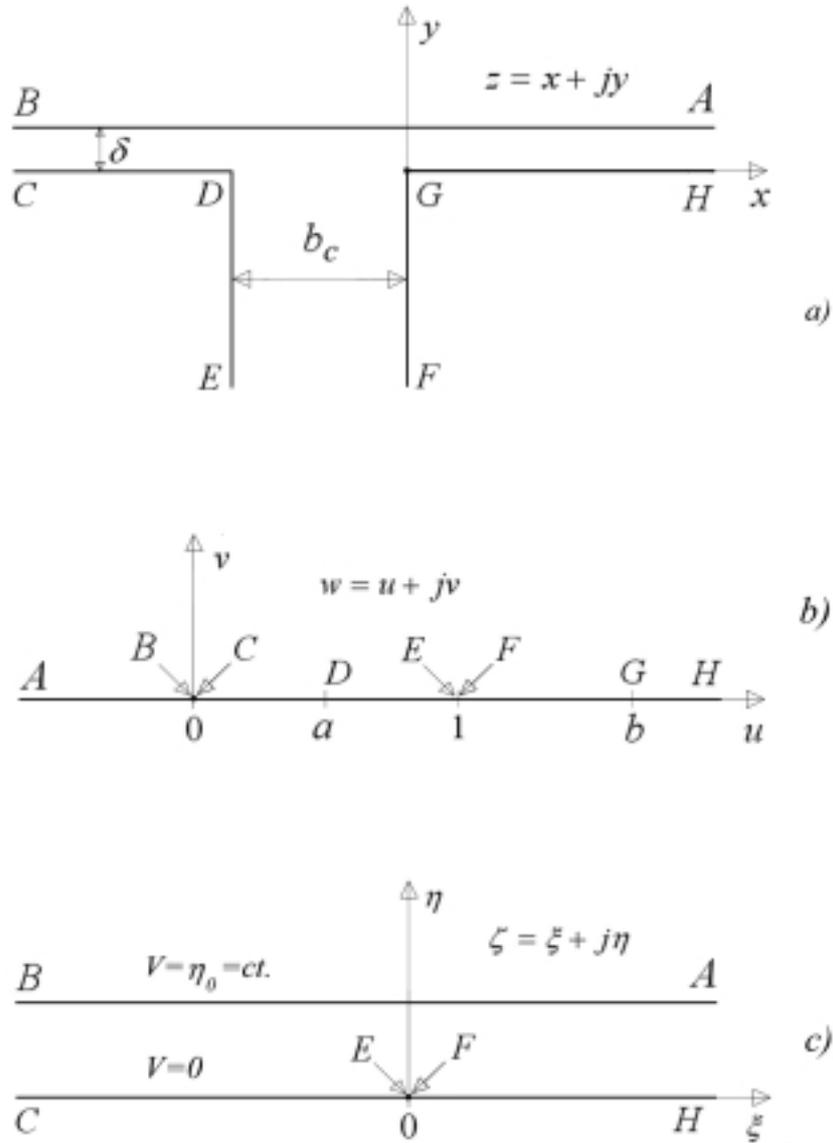
Fig. 4 The conformal mapping of the complex planes: Z, W,  $\zeta$
