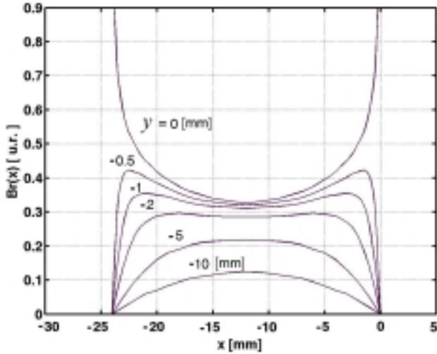
Fig. 5 The distribution of the flux density radial component across the direction of the slot width ( $b_c=24$  mm), near the air gap ( $y=0\dots-10$  mm);  $\delta=5$  mm
