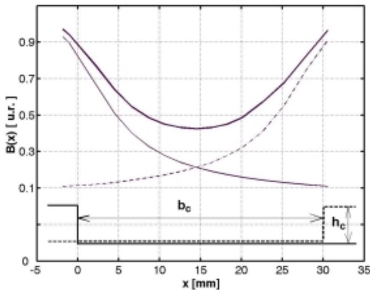
Fig. 2 The superposition method: flux density distribution on the AB boundary, for  $\delta = 5$  mm,  $h_c = 100$  mm and  $0 < x < 30$  mm.
