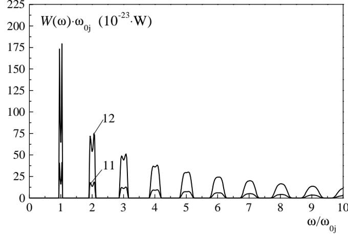
Fig. 7. Spectral distribution of synchrotron radiation power of the electrons moving in a spiral in relativistic case at low harmonics at  $B^{ext} = 10^{-4} \text{ T}$ ,  $V_{\perp vac} = 0.24 \cdot 10^9 \text{ m/s}$  and  $V_{\parallel vac} = 0.15 \cdot 10^8 \text{ m/s}$ ,  $\omega_{0j} = 0.105 \cdot 10^8 \text{ rad/s}$ ,  $r_{0j} = 22.85 \text{ m}$ ,  $j=11,12,\dots,18$ .
