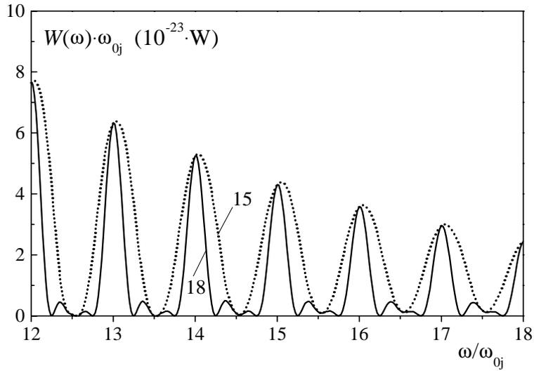
Fig. 14. Spectral distribution of synchrotron radiation power of two electrons moving in a spiral in relativistic case at higher harmonics
