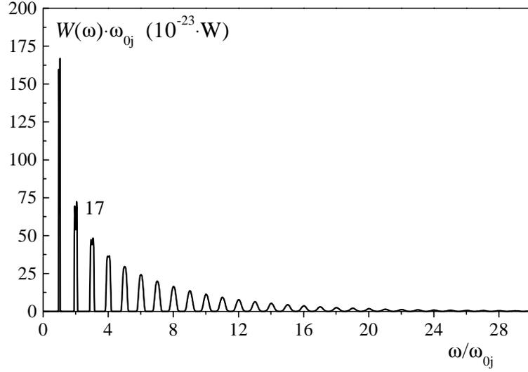
Fig. 11. Spectral distribution of synchrotron radiation power of two electrons moving in a spiral in relativistic case at higher harmonics at  $B^{ext} = 10^{-4}$  T,  $V_{\perp vac} = 0.24 \cdot 10^9$  m/s and  $V_{\parallel vac} = 0.15 \cdot 10^8$  m/s. curve 17 – the time shift  $\Delta t_{12}^{17} = 2\pi/\omega_{017}$  and
