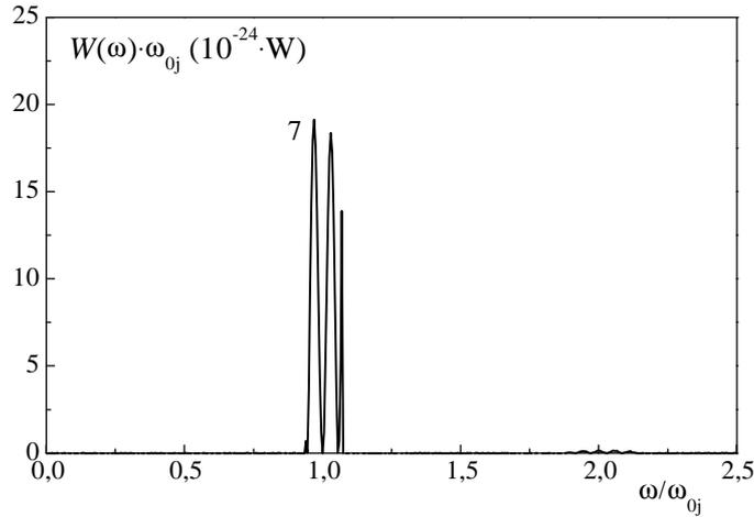
Fig. 5. Spectral distribution of radiation power for two electrons moving in a spiral in non-relativistic case. Curve 7 –
