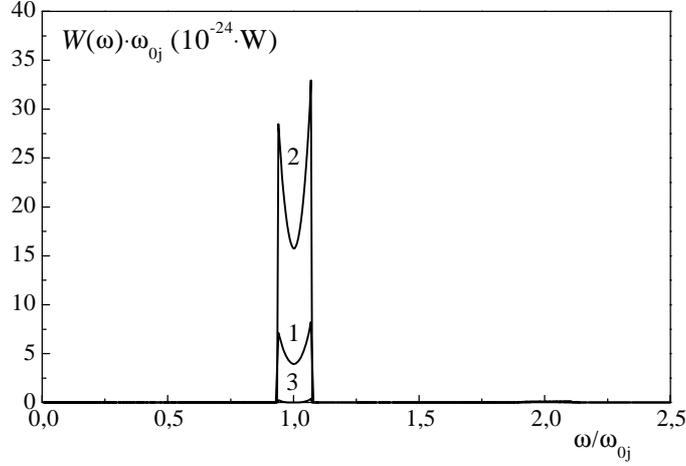
Fig. 1. Spectral distribution of radiation power for the electrons moving in a spiral in non-relativistic case at  $B^{ext} = 10^{-4}$  T,  $V_{\perp vac} = 0.2 \cdot 10^8$  m/s,  $V_{\parallel vac} = 0.2 \cdot 10^8$  m/s,  $r_{0j} = 1.142$  m,  $\omega_{0j} = 0.1751 \cdot 10^8$  rad/s,  $j=1,2,\dots,10$ .
