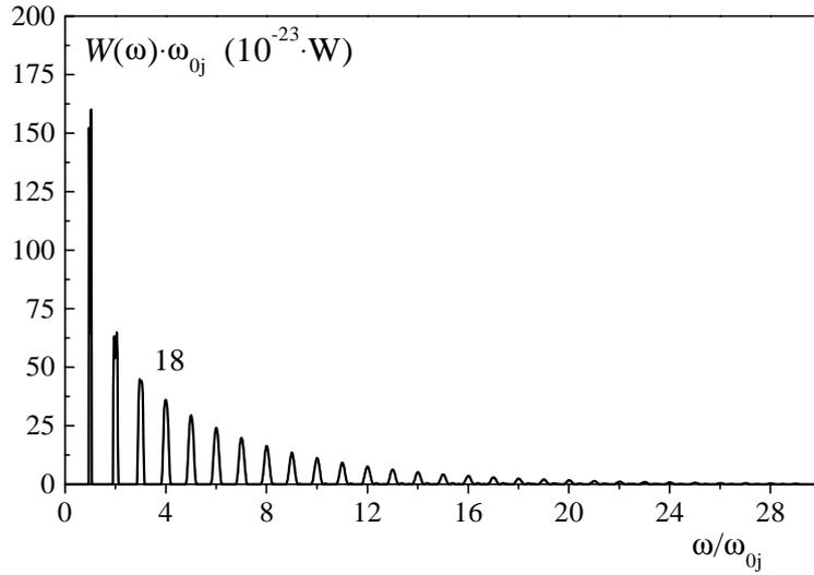
Fig. 13. Spectral distribution of synchrotron radiation power of two electrons moving in a spiral in relativistic case at higher harmonics at  $B^{ext} = 10^{-4}$  T,  $V_{\perp vac} = 0.24 \cdot 10^9$  m/s and  $V_{\parallel vac} = 0.15 \cdot 10^8$  m/s, curve 18 – the time shift  $\Delta t_{12}^{18} = 4\pi / \omega_{018}$  and
