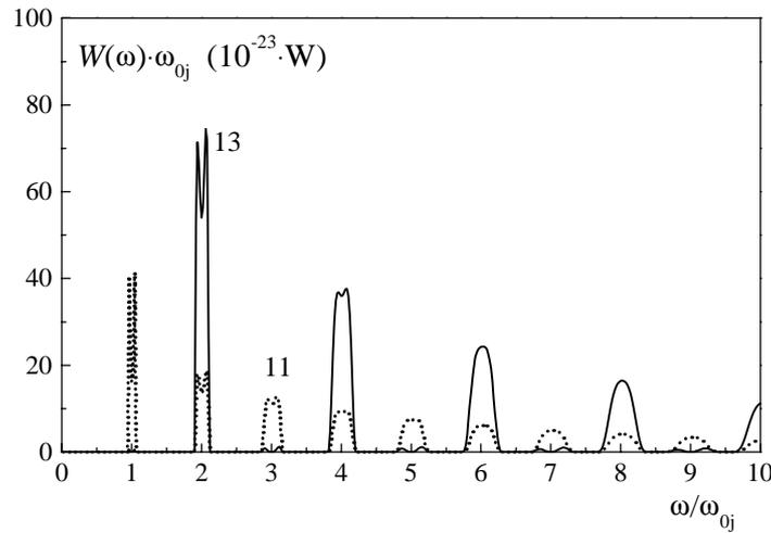
Fig. 8. Spectral distribution of synchrotron radiation power of the electrons moving in a spiral in relativistic case at low harmonics at  $B^{ext} = 10^{-4} \text{ T}$ ,  $V_{\perp vac} = 0.24 \cdot 10^9 \text{ m/s}$ ,  $V_{\parallel vac} = 0.15 \cdot 10^8 \text{ m/s}$ . Curve 11 – a single electron with  $P_{vac11}^{int} = 0.2092 \cdot 10^{-21} \text{ W}$ ,
