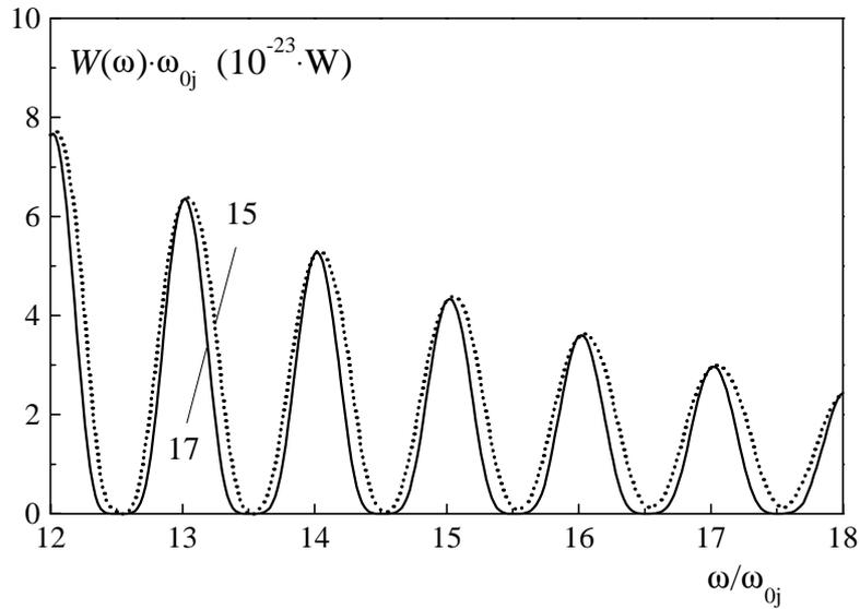
Fig. 12. Spectral distribution of synchrotron radiation power of two electrons moving one by one in a spiral at higher harmonics.
