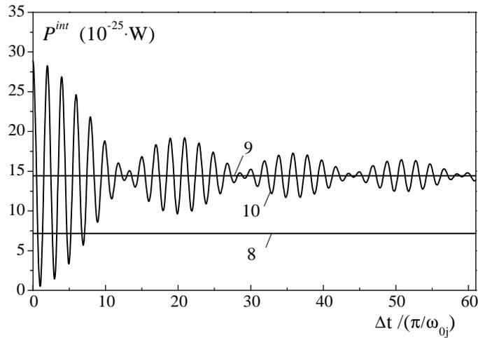
Fig. 6. Radiation power in dependence on time shift between two electrons moving in a spiral in non-relativistic case at  $V_{\perp vac} = 0.2 \cdot 10^8$  m/s and  $V_{\parallel vac} = 0.2 \cdot 10^8$  m/s. Radiation power of a single electron (curve 8). Radiation power of two separate electrons (curve 9). Radiation power of two electrons moves one by one depending on their location in a spiral (curve 10).
