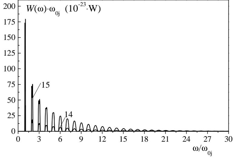
Fig. 9. Spectral distribution of synchrotron radiation power of the electrons moving in a spiral in relativistic case at higher harmonics at  $B^{ext} = 10^{-4}$  T,  $V_{\perp vac} = 0.24 \cdot 10^9$  m/s,  $V_{\parallel vac} = 0.15 \cdot 10^8$  m/s. Curve 14. – a single electron with
