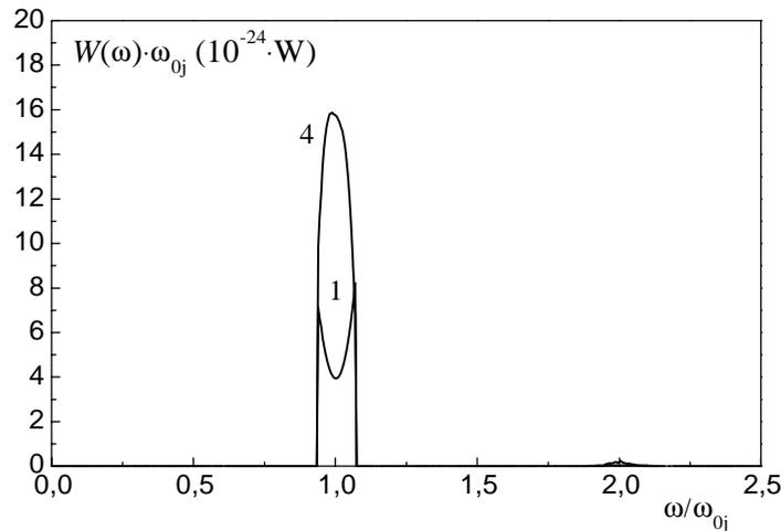
Fig. 2. Spectral distribution of radiation power for the electrons moving in a spiral in non-relativistic case. Curve 1 – the radiation spectrum of a single electron. Curve 4 – two electrons at  $\Delta t_{12}^4 = 10\pi / \omega_{04}$  and  $P_{vac4}^{int} = 0.1848 \cdot 10^{-23}$  W.
