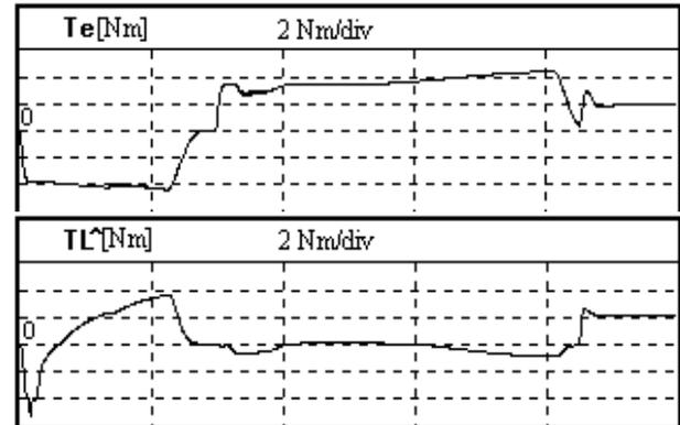
Fig. 10. Transient responses for  $\omega^* = \pm 400$  rpm, detuned case:  $J = 5J_o$ ,  $R = 1.2R_o$ ,  $\lambda_0 = 0.9\lambda_{0o}$ .
