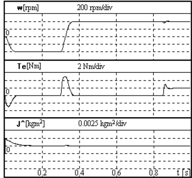
Fig. 9. Transient responses for  $\omega^* = \pm 400$  rpm,  $J = 0.5 J_o$ .
