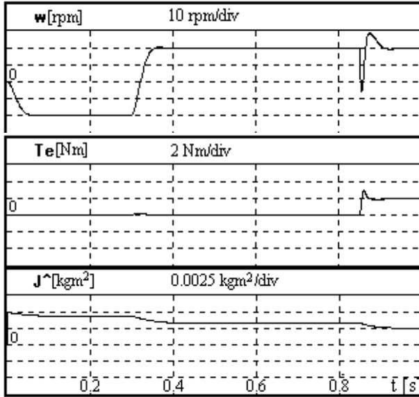
Fig. 7. Transient responses for  $\omega^* = \pm 20$  rpm,  $J = 0.5 J_o$ .
