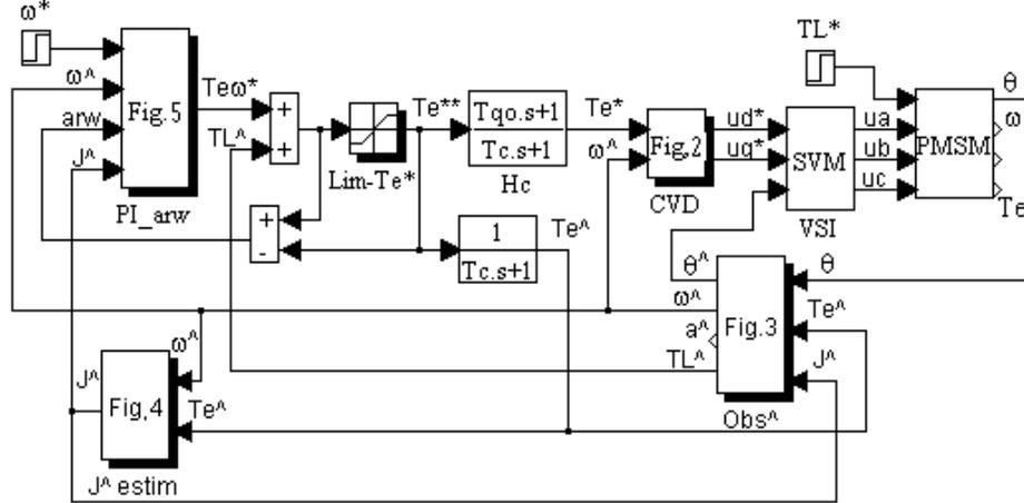
Fig. 1. Structure of current sensorless speed-torque control based on adaptive observer and inertia identification.
