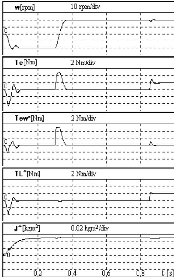
Fig. 6. Transient responses for  $\omega^* = \pm 20 \text{ rpm}$ ,  $J = 10 J_o$ .
