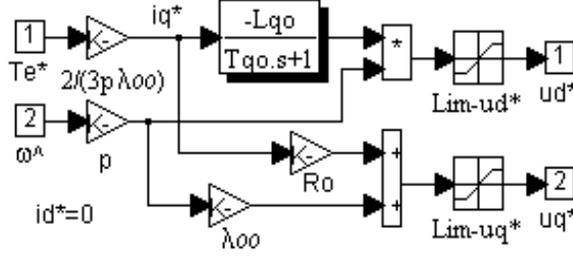
Fig. 2. Current to voltage decoupling. PMSM torque control with  $i_d^* = 0$ .
