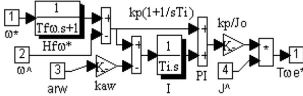
Fig. 5. Speed controller PI anti-windup with reference filter and inertia adaptive.
