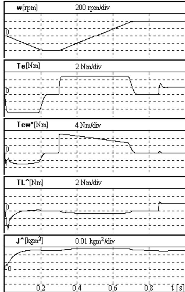
Fig. 8. Transient responses for  $\omega^* = \pm 400 \text{ rpm}$ ,  $J = 5 J_o$ .
