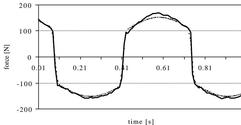
Fig. 4a. Force vs. time for 0.06 A \_\_\_\_\_ experimental; ..... predicted
