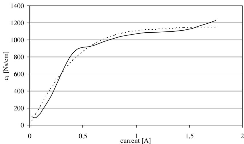
Fig. 7. The parameter  $c_1$  vs. current  $u$ , experimental ( — ) and predicted ( ... )
