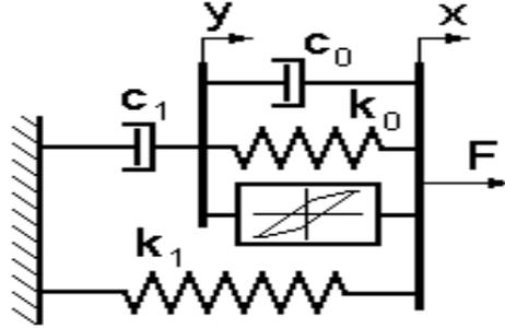
Fig. 3. Bouc-Wen modified mechanical model
