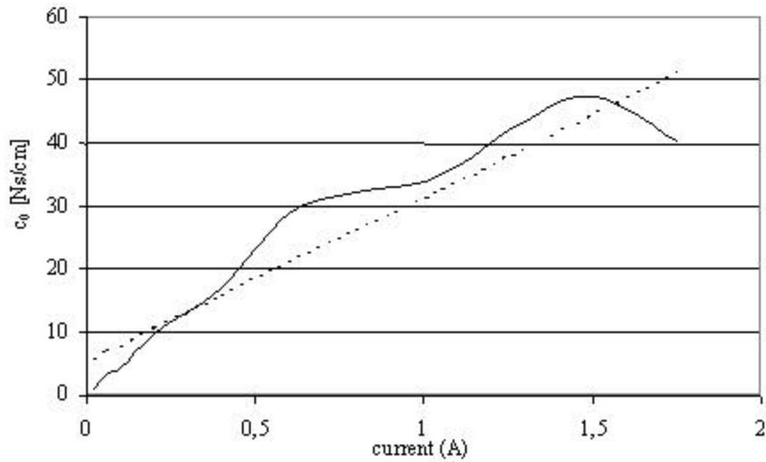
Fig. 6. The parameter  $c_0$  vs. current  $u$ , experimental ( — ) and predicted ( ... )
