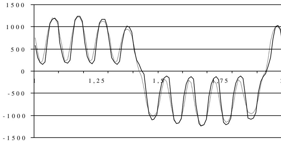
Fig. 10b. Force [N] versus time [s] in the second test case \_\_\_\_\_ experimental; ..... predicted
