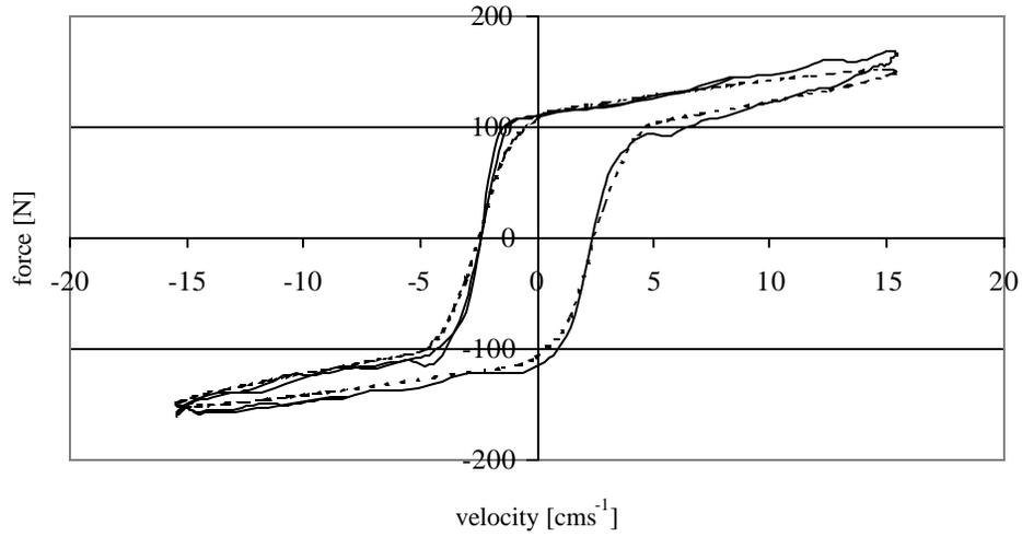
Fig. 4b. Force vs. velocity for 0.06 A \_\_\_\_\_ experimental; ..... predicted
