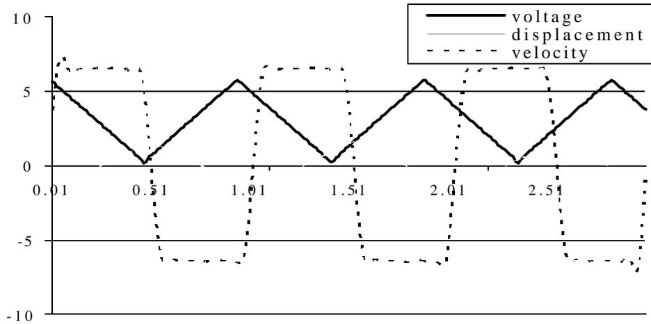
Fig. 11a. The voltage [volts], displacement [cm] and velocity [cm/s] for the third test case
