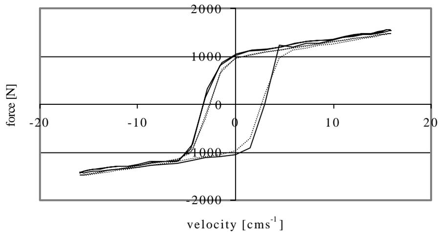
Fig. 5b. Force vs. velocity for 1.75 A \_\_\_\_\_ experimental; ..... predicted
