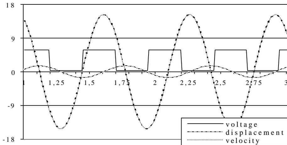
Fig. 9a. Time histories of the voltage [volts], displacement [cm] and velocity [cm/s] in the first test case
