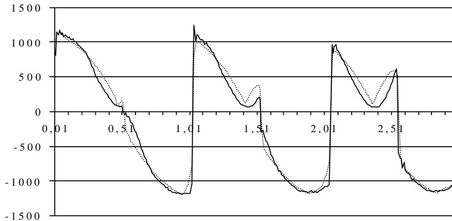
Fig. 11b. Force [N] versus time [s] in the third test case \_\_\_\_\_ experimental; ..... predicted
