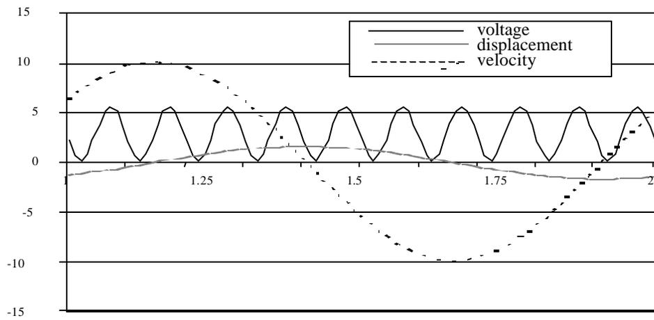
Fig. 10a Time histories of the voltage [volts], displacement [cm] and velocity [cm/s] in the second test case
