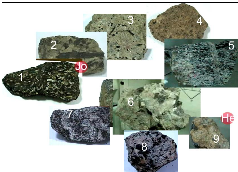
Figure 3. The main type of rocks from DAM: 1, hornblendite; 2, diorite; 3, syenite; 4, granite; 5, oriented nephelin syenite; 6, nepheline syenite; 7, essexite; 8, monzodiorite; 9, syenite with paragonite; Jo–Jolotca, He–Hereb.
