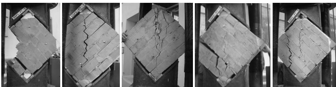
Fig. 8 Failure modes of pretension rods (PT) applied on one side and both sides
