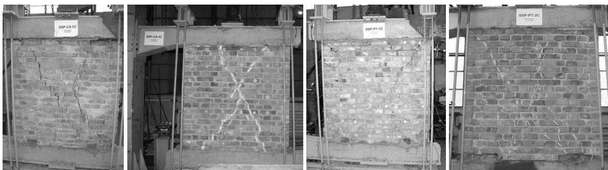
Fig. 12 – Failure modes for cyclic specimens reinforced with CA and PT on one and both sides.
