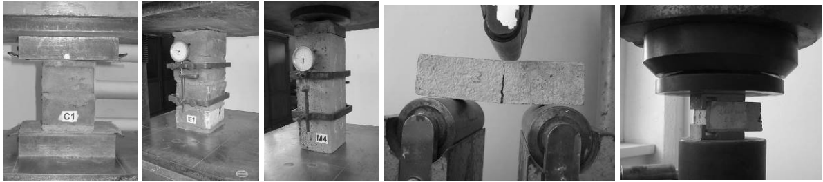
Fig. 2 – Tests on masonry and components (mortar and brick).
