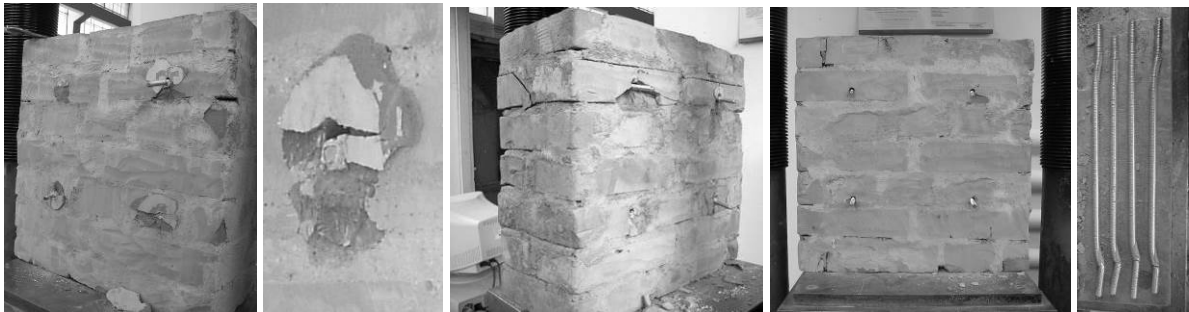
Fig. 4 – Failure modes for chemical anchor (CA) and steel rods (PT) connections.
